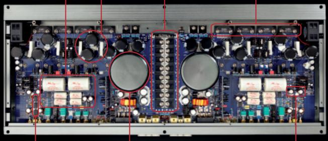
Our amplifiers are featured with IC OPAMP Analog device by Burr Brown Toroid is designed to comprehend with audio signal while the Toroid Protection helps with the circuit
